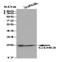
Western blot analysis of CD63 in Jurkat lysates using CD63 antibody.
