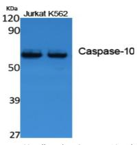
Western Blot analysis of extracts from Jurkat, K562 cells, using Caspase-10 Polyclonal Antibody.. Secondary antibody was diluted at 1:20000
